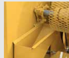
Internally Lubricated Packing Gland with Drip Catch Pan
